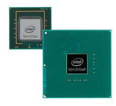
GMA 500 to communicate directly to a flat-panel display. The LVDS interface supports 18-bit or 24-bit color and EDID and EDID-less displays with a maximum pixel clock of 112 MHz. SDVO may be used for any external display device such as HDMI/DVI, analog TV, VGA/CRT and LVDS, and includes EDID and EDID-less support with a 160 MHz pixel clock.
